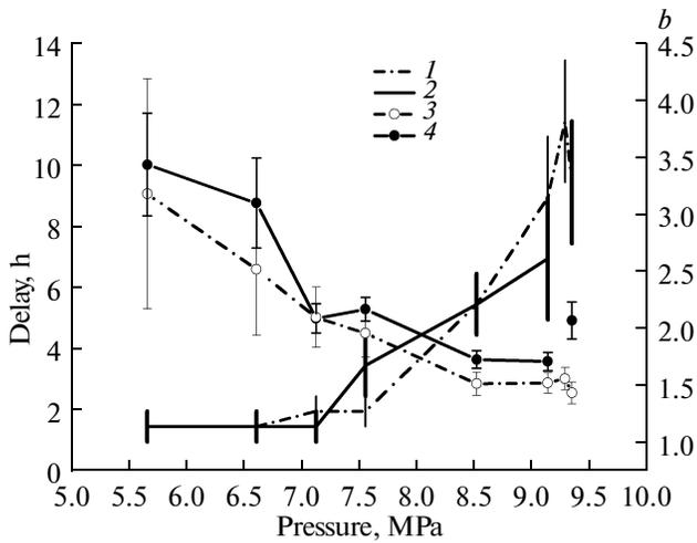
**Fig. 21.** Delay in the response and the slope of the frequency-magnitude curve  $b$  depending on water pressure based on the data from the entire catalogue and multiplets. Delay: (1) inferred from the entire catalogue, (2) inferred from the catalogue of multiplets; the slope of the frequency-magnitude curve: (3) inferred from the entire catalogue, (4) inferred from the catalogue of multiplets.
