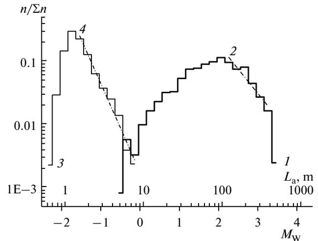
Fig. 20. The size distribution of heterogeneities (1) and the magnitude distribution of earthquakes (3), (2) power-law approximation of the descending branch of the size distribution of heterogeneities, (4) the Gutenberg–Richter law approximation of the earthquakes distribution.
