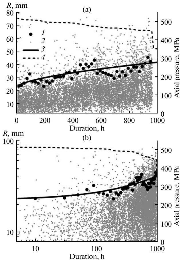
**Fig. 23.** The size of the cloud of seismicity as a function of time from the commencement of nucleation on the linear (a) and logarithmic (b) scales: (1) size of the cloud estimated from the gyration radius, (2) distance between the center of nucleation and the hypocenters of the acoustic events, (3) power-law approximation of the size of the cloud (the initial size of the nucleation “embryo” taken into account), (4) axial stress provided by the press.
