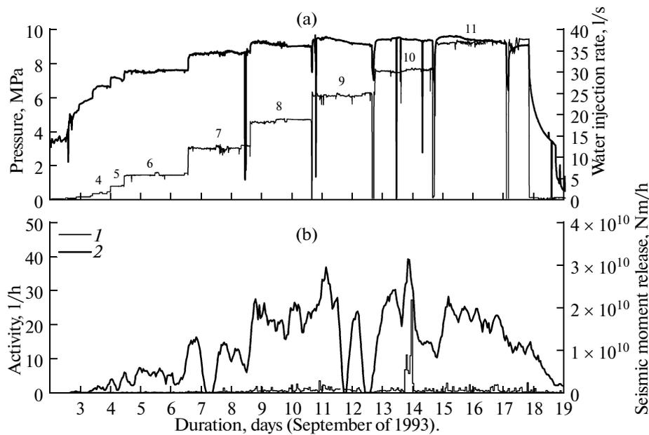
**Fig. 12.** History of water injection in the natural experiment: (a) water injection rate ( $I$ ) and pressure excess in the hole over the formation pressure (differential pressure) (2). Numbers of series used in this work are indicated near the curve of the water injection rate. (b) Parameters of induced seismicity: (1) activity (number of seismic events per hour), (2) rate of the seismic moment release.
