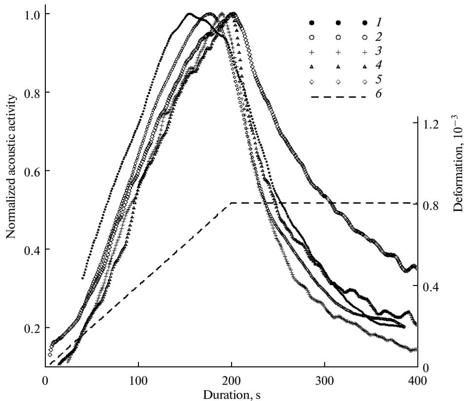
Fig. 5. Normalized curves of acoustic activity under different acting differential stresses and the initiating step of deformation (experiment SS70): (1) 30 MPa, (2) 55 MPa, (3) 105 MPa, (4) 155 MPa, (5) 215 MPa, (6) initiating step of deformation.
