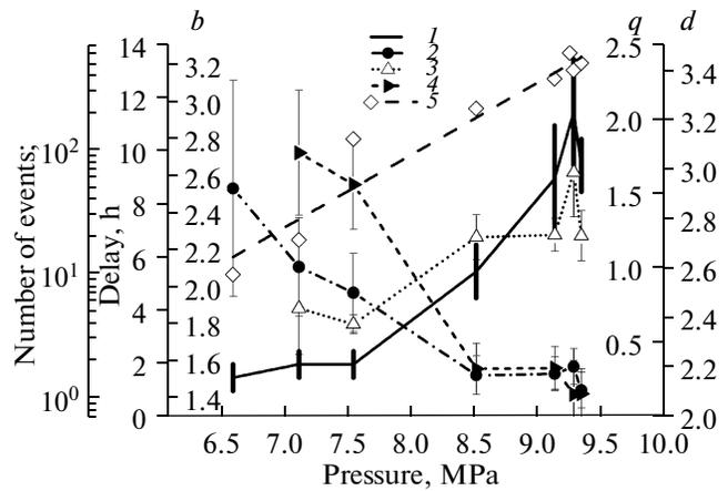
**Fig. 17.** Parameters of the seismic regime depending on the pressure of injected water: (1) delay in the maximum activity, (2) the slope of the frequency-magnitude plot, (3) fractal size of the set of hypocenters, (4) parameter *q*, (5) total number of earthquakes in series; the straight line corresponds to the exponential approximation.
