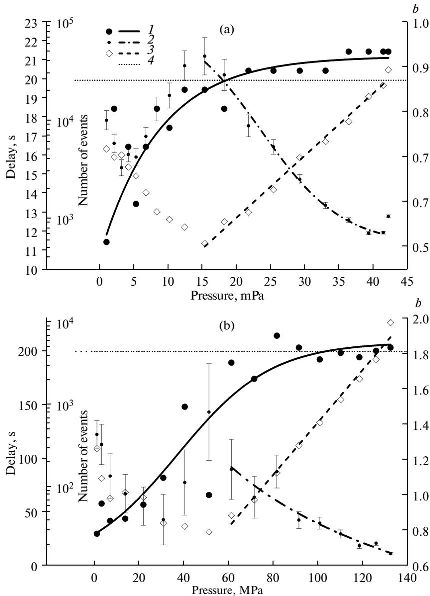
**Fig. 3.** Parameters of the acoustic regime with different acting stresses: (a) experiment A52, (b) experiment A62: (1) delay in maximum activity relative to the beginning of initiation, (2) slope of the frequency-magnitude curve, (3) number of events in each series (the straight line corresponds to exponential approximation), (4) the duration of the increase of the initiating step: 20 s in A52 and 200 s in A62.
