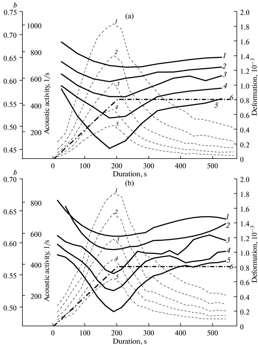
**Fig. 7.** The slope of the frequency-magnitude curve in the series: (a) experiment SS40: (1) 140 MPa, (2) 152 MPa, (3) 163 MPa, (4) 173 MPa, (5) 182 MPa, (b) experiment SS70: (1) 180 MPa, (2) 191 MPa, (3) 202 MPa, (4) 211 MPa, (5) 220 MPa. The dashed line indicates corresponding curves of acoustic activity. (6) initiating step of deformation.
