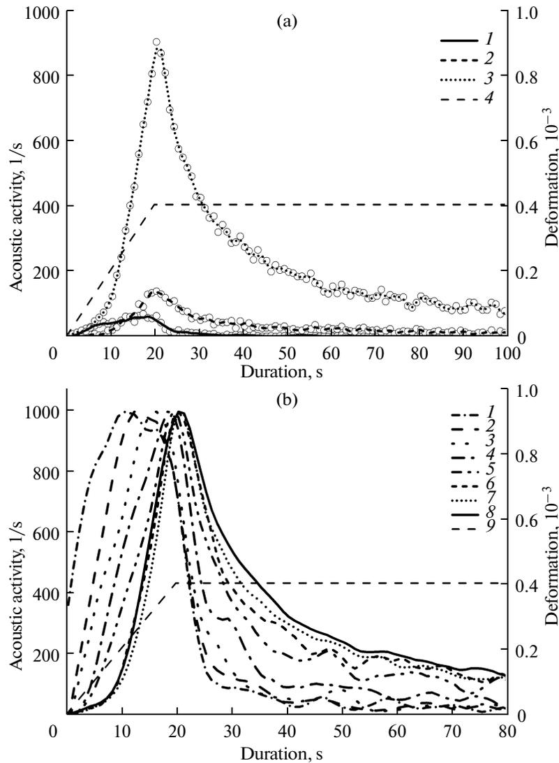
**Fig. 2.** Acoustic activity in the experiment A52: (a) examples of initial data (points) and smoothed curves corresponding to different values of acting stresses: (1) 8.3 MPa, (2) 29.2 MPa, (3) 41.3 MPa, (4) initiating step of deformation; (b) normalized curves of acoustic activity under different acting stresses: (1) 1.0 MPa, (2) 5.3 MPa, (3) 10.2 MPa, (4) 15.3 MPa, (5) 21.7 MPa, (6) 29.2 MPa, (7) 39.2 MPa, (8) 42.1 MPa, (9) initiating step of deformation.
