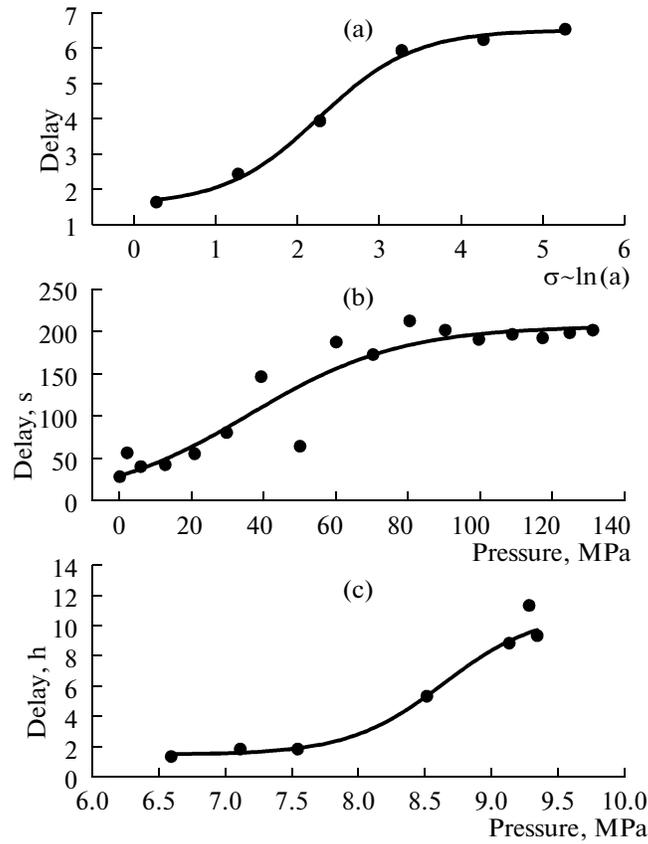
**Fig. 25.** Dependence of the delay in the commencement of relaxation on the acting stresses; (a) mathematical model, (b) laboratory experiment, (c) natural experiment in Soultz-sous-Forêts.
