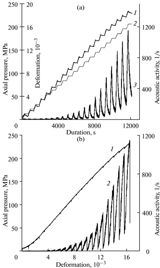
**Fig. 4.** Loading history and loading curve for Specimen SS70: (a) loading history: (1) axial stress, (2) axial deformation, (3) acoustic activity; (b) loading curve: (1) stress–strain diagram, (2) acoustic activity.
