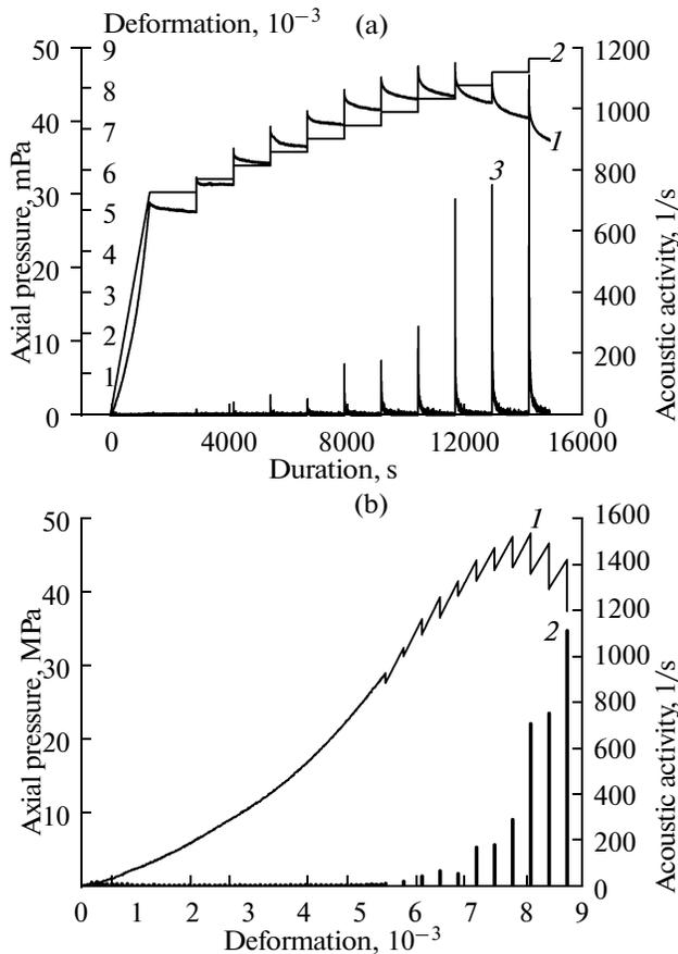
**Fig. 8.** Loading history and loading curve for Sample A42: (a) loading history: (1) axial stress, (2) axial deformation, (3) acoustic activity; (b) loading curve: (1) stress–strain diagram, (2) acoustic activity.
