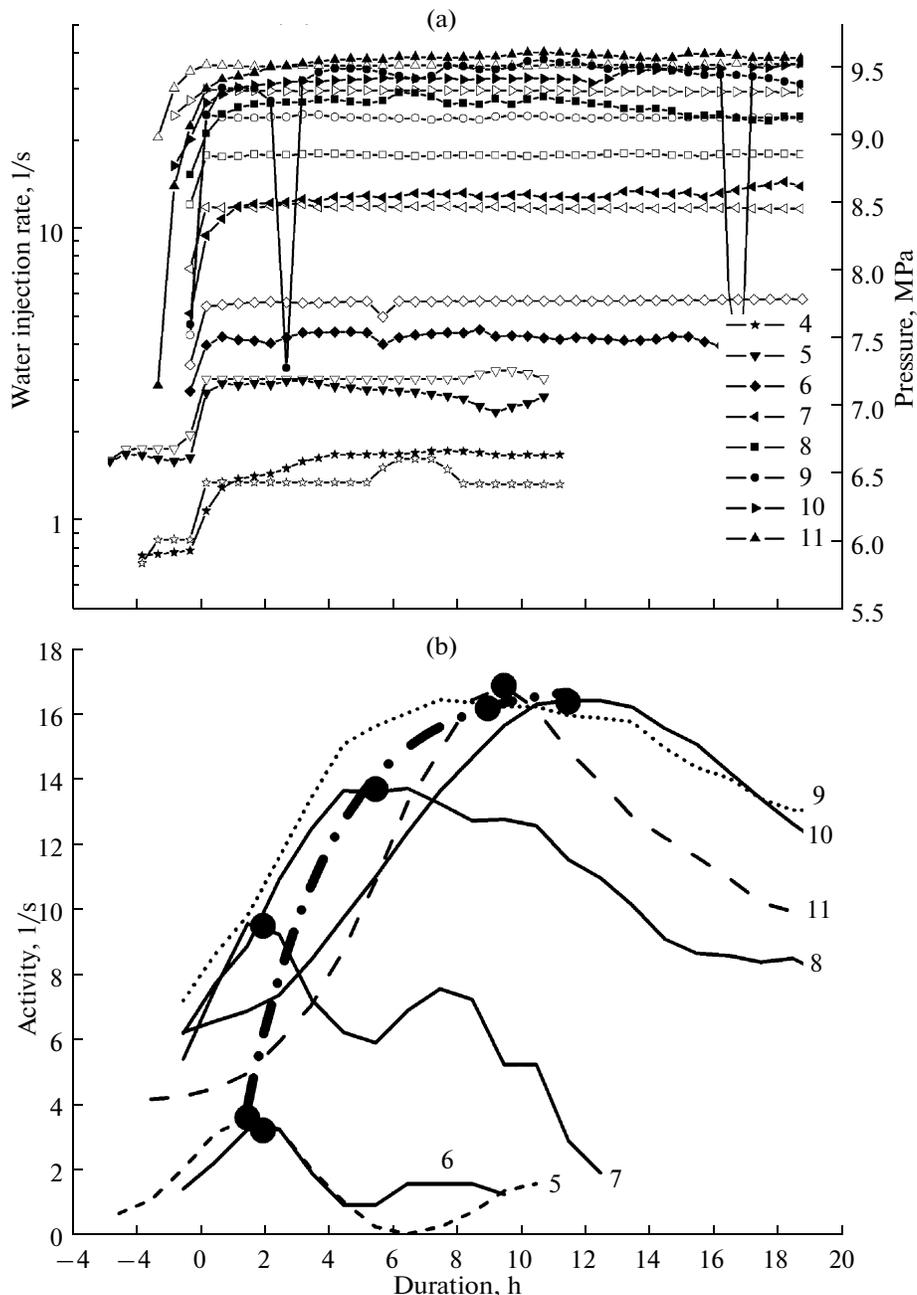
**Fig. 16.** Water injection and seismic activity in the natural experiment: (a) variations in the water injection rates (open symbols) and differential pressure (solid symbols) for different series. Numbers of curves correspond to the series numbers; (b) variations in the seismic activity for different series based on selected data (series numbers are indicated near the curves). Solid dots indicate the maxima in seismic activity for each series.
