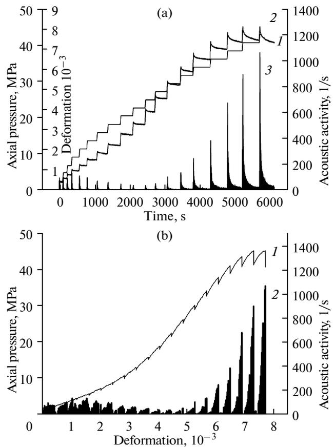
**Fig. 1.** Loading history and loading curve for Specimen A52: (a) loading history: (1) axial stress, (2) axial strain, (3) acoustic activity; (b) loading curve: (1) stress–strain diagram, (2) acoustic activity.
