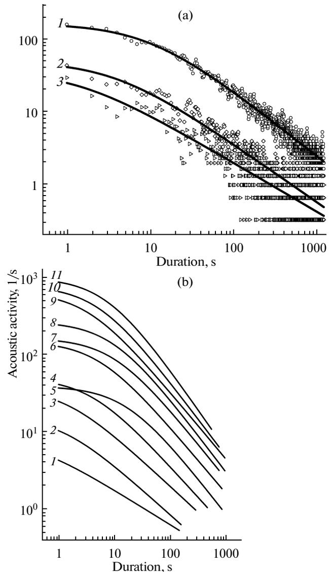
**Fig. 9.** Acoustic activity in experiment A42: (a) examples of initial data (points) and approximation by the Omori's law
