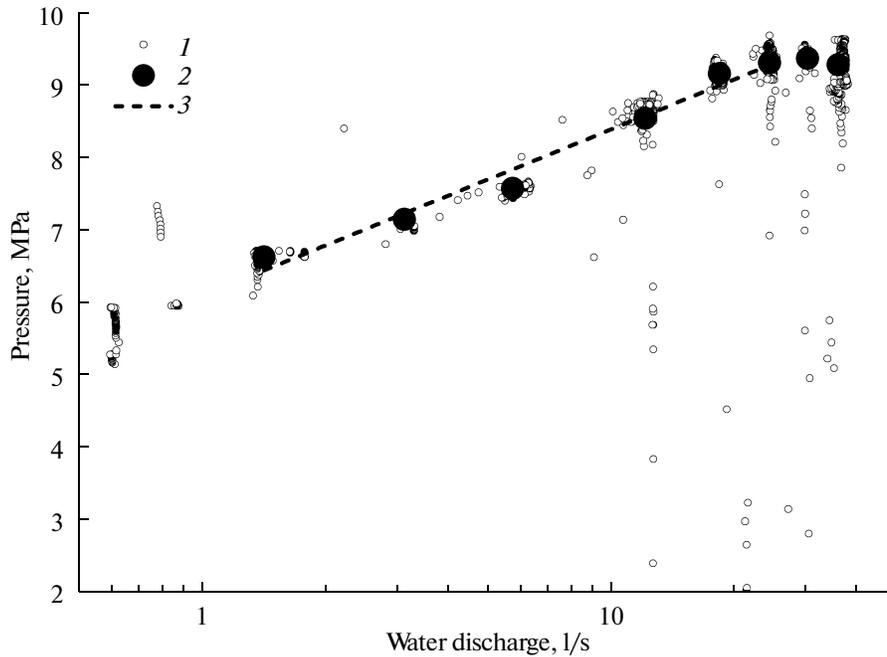
Fig. 13. Water injection rate and pressure: (1) initial data, (2) average over series, (3) approximation  $Q \sim e^{\beta P}$ .
